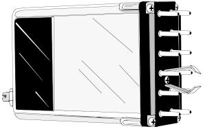
The Series 236, 237 and 238 Time Delay Relays consist of a standard 219 industrial relay and a solid state timing module to provide delayed transfer of relay contacts after application of power or activation of control switch. The relay and timing module are enclosed in a flame resistant polycarbonate cover.
